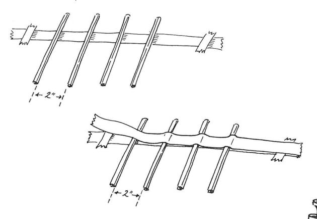
Next, insert the three-inch nails into each open end of the straws. They will have a tendency to slip out easily. You can prevent this from happening by first sliding a paper clip into both ends of the straws and then sliding the nail next to the paper clip as shown in the drawing.
