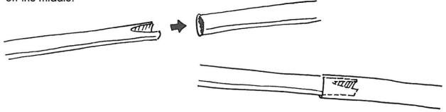
Place a straw segment about twelve inches from one end of the tape on the floor. Center this segment by placing it on the middle mark. Press down firmly so that the straw sticks to the tape. Place another straw 2 inches from the first straw segment. Center it and press down firmly. Continue to add straw segments in this manner until you reach a point about 10-12 inches from the other end of the tape.
