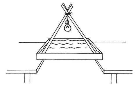
Connect the two wires from the light bulb to the two wires from the battery holder. Darken the room. Wiggle your finger on the surface of the water. If all is working well, you should see a pattern of shadows on the floor. A large white sheet of paper placed under the tank will make these shadows more visible.
