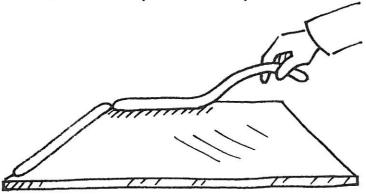
Test the seal between the clay and plastic by adding water to the enclosure until a pool 1/4 inch deep is obtained. Look for any leaks. Work the clay at those spots which are leaking, until all are fixed.
